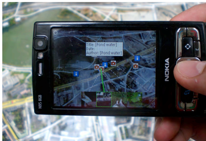
Figure 12. The MapLens application: augmenting a physical map with a handheld AR view [50].
