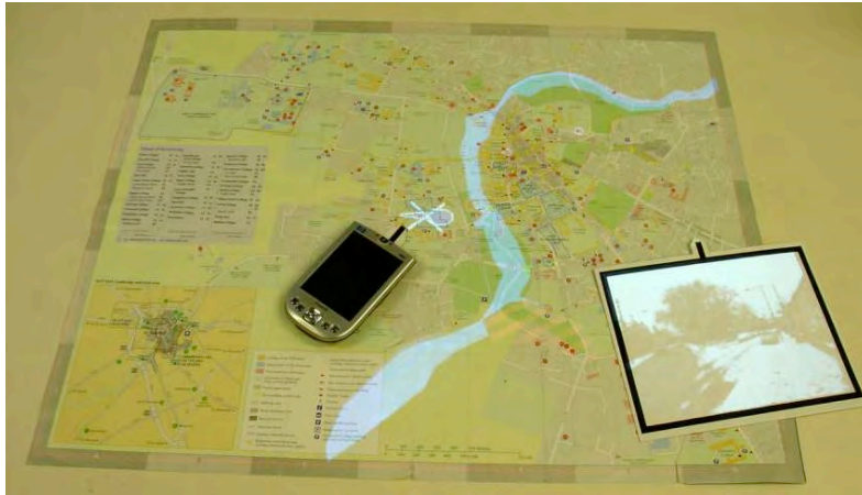
Figure 11. An Augmented Map using Projection technology and supporting tracking of physical objects. Image Courtesy of Gerhard Reitmayr [40].
