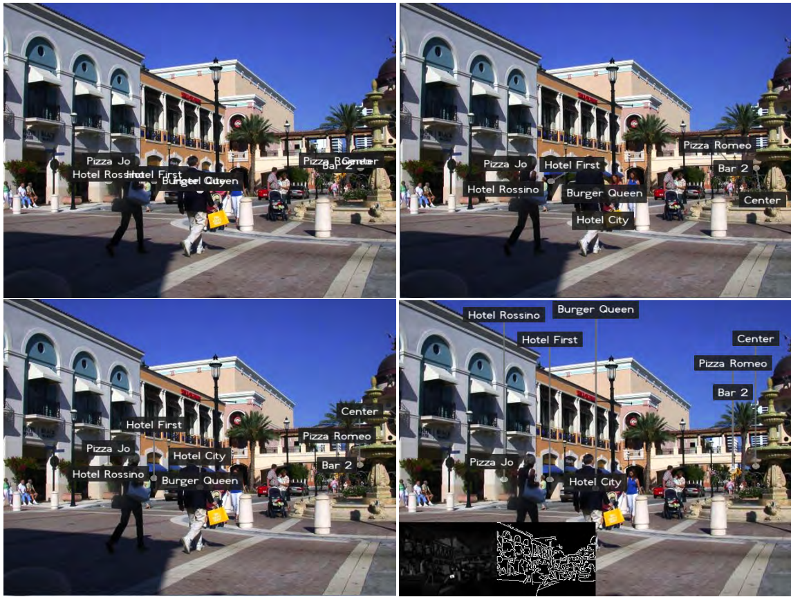
Figure 12: Comparison of layout techniques (left to right): naive, height separation, planar separation, our approach with top placement.
