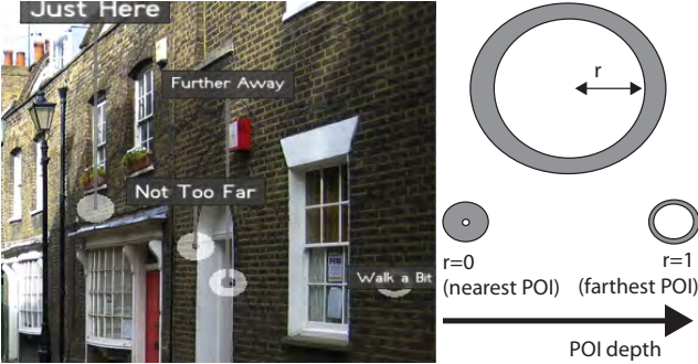
Figure 7: Anchor Ring concept and example with POIs at different distance.
