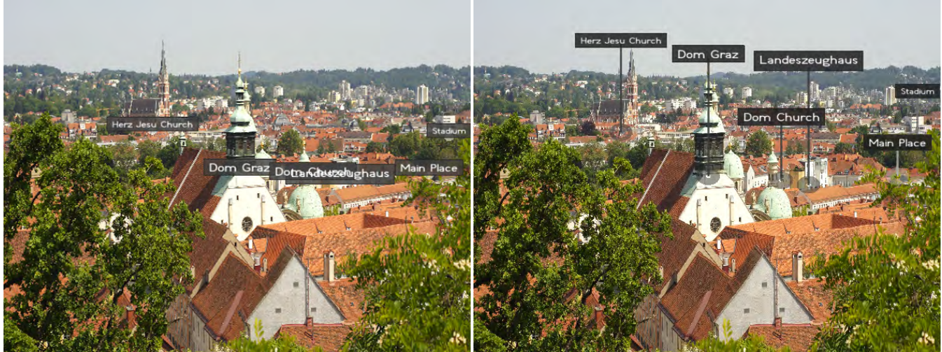
Figure 1: Common labeling as used in many AR browsers (Left) compared to our image-based approach (Right). Position of the labels can be automatically optimized, but also their appearance, including depth cue for the labels' anchor or their leader lines.
