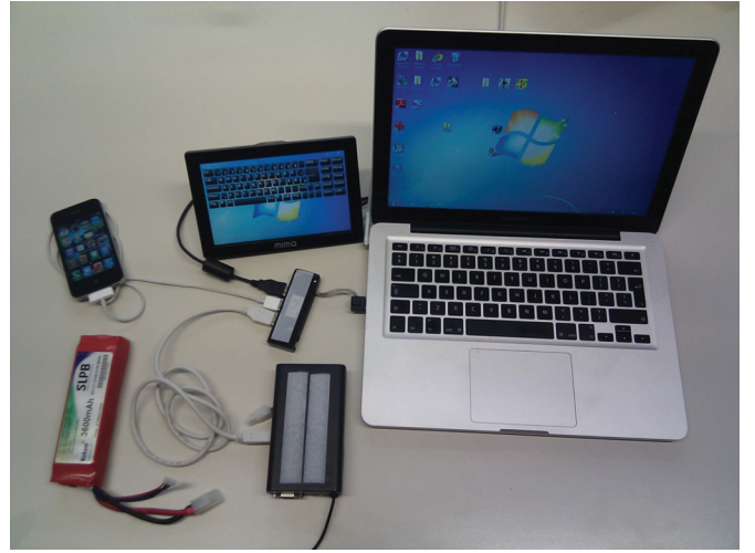
Fig. 3. Hardware setup in detail. Apple iPhone 4s , Mimo Touch 2 , Battery Pack and Novatel GPS receiver, connected via USB hub to an Apple MacBook Pro .
