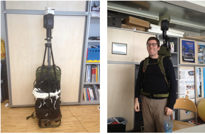
Fig. 2. Left: data acquisition system, consisting of the backpack, the Point Grey Ladybug 3 camera mounted on a tripod and the antenna of the Novatel GPS receiver on top of the camera. Right: a user operating the acquisition system.
