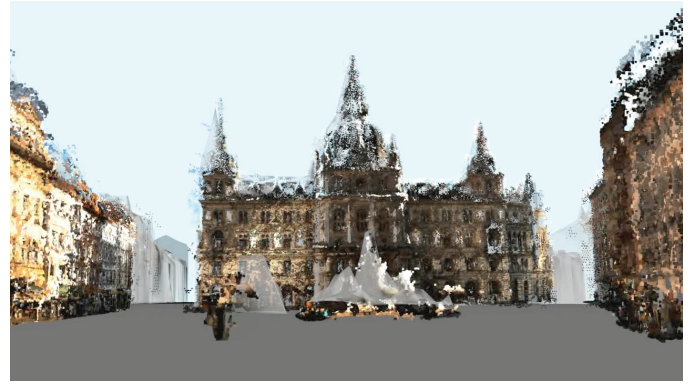
Fig. 6. Exemplary view of a reconstruction of the Grazer Hauptplatz using PMVS [6]. Since the models are registered, the point cloud accurately aligns with the polygonal building models visualized in light grey color.
