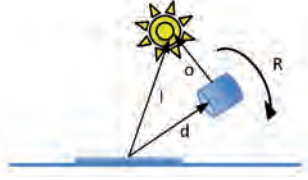
Figure 2: With the LED light source in a fixed configuration to the camera, there are only 3 degrees of freedom in the input to the SVBRDF function.
