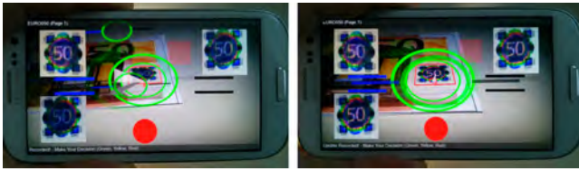
Figure 15: Improved user interface (left): Top-left patch showing reference data for the nearest reference view, top-right patch showing captured data by the user. Bottom-left patch showing live view of the warped hologram patch. Additional elements represent visual ranges for easier alignment. Automatic recapture (right): The hologram is re-captured when a more suitable pose is encountered.
