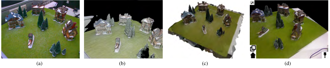
Figure 3: Scene Representation. Our system works independently of the scene capturing technology or rendering representation. The real scene shown in (a) can be reconstructed and rendered using different methods, such as (b) rendering colored voxels of a volumetric representation generated with KinectFusion, (c) rendering a polygonal mesh of a reconstruction or (d) image based rendering of a reconstructed proxy mesh.
