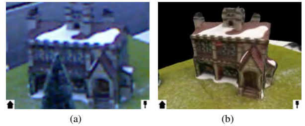
Figure 10: Scene Zooming Methods. (a) A pure digital zoom causes artifacts in the video image. (b) We zoom into a virtual representation, which provides close-up views with higher resolution.
