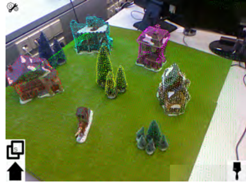
Figure 5: Scene Segmentation. We automatically segment the scene to identify the ground plane defining the world coordinate system and single objects on the ground plane. We use this knowledge to control the viewpoints of transitions. Colors represent the segmented object.
