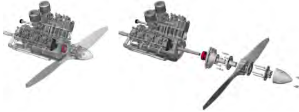
(b) Explosion diagram for extracting the highlighted part from an engine.
