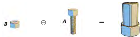
Figure 4: Creation of a C -Space obstacle. Calculating the Minkowski difference B \ominus A yields the inflated obstacle \mathcal{A}_B .
