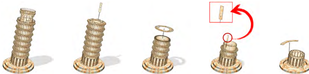
Figure 1: Key frames from a disassembly sequence for the Leaning Tower CAD model. Our approach identifies reusable blocking information and evaluates the geometric feasibility of part removals in parallel. Thus, we are able to create disassembly sequences for models such as this 4,193 part assembly within minutes instead of days. Furthermore, unstable configurations are avoided by using structural constraints to elevate reproducibility on real-world objects. We facilitate the visual assessment of sequences by combining previewing techniques with visual cues to highlight smaller details.
