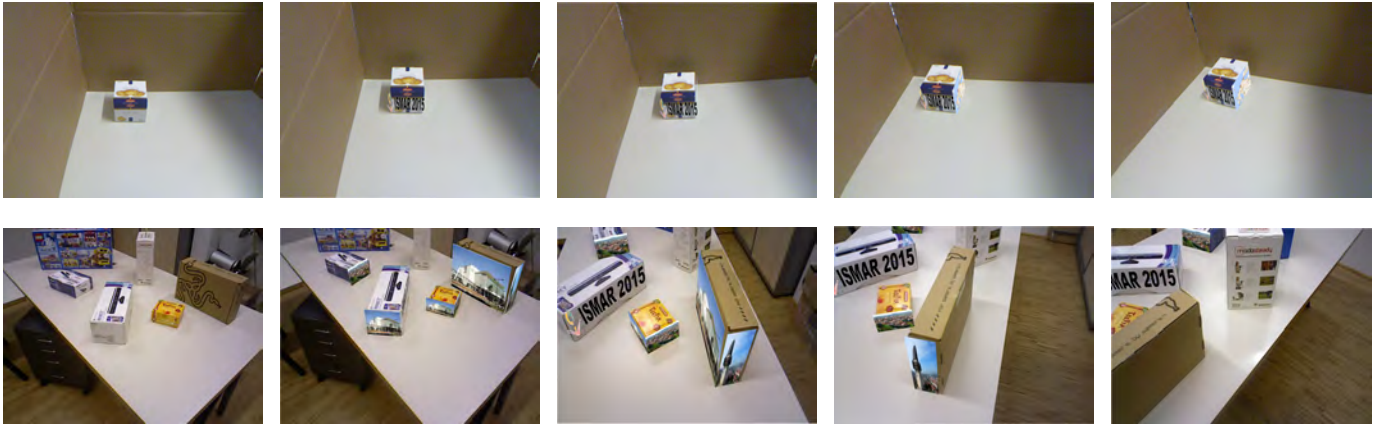
Fig. 11: Simple AR application. We render virtual content on rectangle surfaces in the scene, as shown from different view points. Top: Tracking and augmenting a single box. Bottom: Tracking and augmenting multiple boxes simultaneously.
