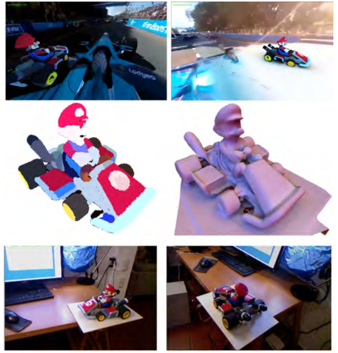
Figure 7: Augmented Virtuality. (top) We place the scan inside a 360° video and relight the geometry using our material estimated and an estimation of lighting in each video frame video. (bottom) Input data and estimated albedo color and lighting.
