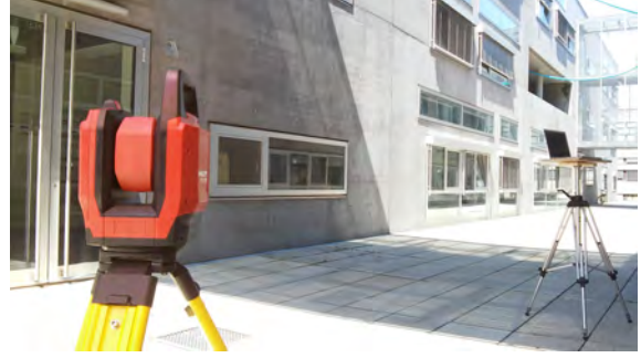
Figure 3: Robotic Total Station and mobile PC used in our experiments. The communication between the devices is done wirelessly over WLAN.
