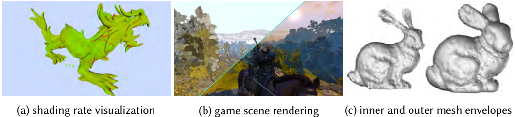
Fig. 1. To evaluate the effectiveness and performance of our on-the-fly vertex reuse strategies, we have implemented a variety of test applications. (a) Visualization of the shading rate achieved during shading of the vertices of a triangle mesh (green vertices are shaded only once, red vertices six or more times). (b) A full rasterization pipeline rendering scene geometry captured from the video game The Witcher 3: Wild Hunt . (c) In general, many geometric algorithms can benefit from vertex reuse, such as the simplification envelopes algorithm shown here. The Witcher 3: Wild Hunt screenshot courtesy of CD PROJEKT S.A.; used with permission.
