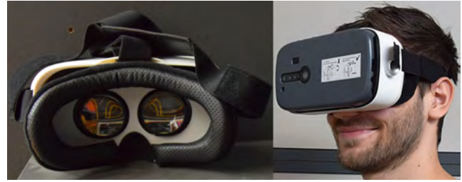
Fig. 9. Untethered smartphone-based headset prototype based on the Qualcomm Snapdragon™ 835 Mobile Platform, with a resolution of 2560 \times 1440 , displaying a stereo view of the Robot Lab scene.
