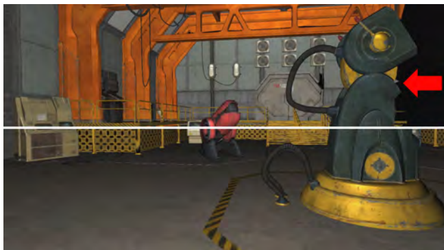
Fig. 3. (top) Image-based rendering methods typically suffer from artifacts caused by disocclusions (red arrow), when the viewpoint is translated. (bottom) SAS can avoid artifacts by predicting future viewpoints and rendering all geometry in the corresponding potentially visible set.
