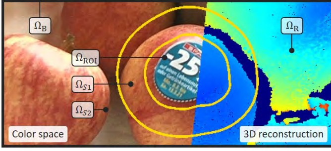
Fig. 2. Regions to define the keyframe suitability criteria. Within the FOV, we distinguish ROI and its surrounding areas as \Omega_{ROI} and \Omega_S , respectively. Further, we separate \Omega_S into \Omega_{S1} and \Omega_{S2} , which denote boundary pixels of ROI with a margin, and the rest, respectively. \Omega_B is a margin surrounding the FOV. The colored points represent areas \Omega_R where scene reconstruction is completed.
