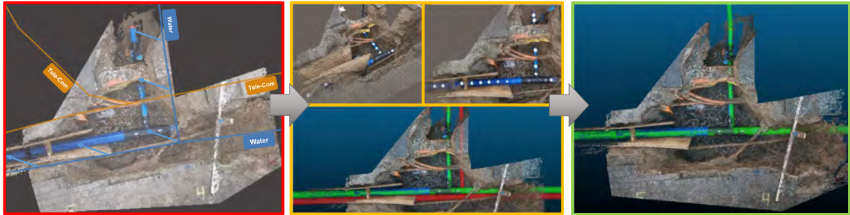
Figure 1: Left: top-down view of a 3D point cloud reconstruction with inaccurate SUE data visualized for different infrastructure types as simple line strings. Middle: Segmentation results from virtual cameras (top), highlighting inaccurate (red) and aligned (green) infrastructure data. Right: fitted 3D infrastructure model shown on a top-down view of a 3D point cloud reconstruction.
