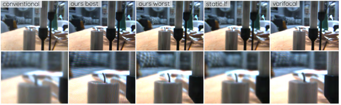
Fig. 12: Through-the-lens photographs of Scene (c) for various display types. We focused the camera at the ground-truth focus distance of 3 dpt (corresponding to the candle in the front). The eye tracking error is 0.6 dpt. The bottom row shows magnified insets of the capturings. Overall, the through-the-lens images confirm the simulated results. While “ours best” leads to the image with best contrast, “ours worst” still manages to outperform the other display types by a small margin. As expected, the conventional display yields the worst results.
