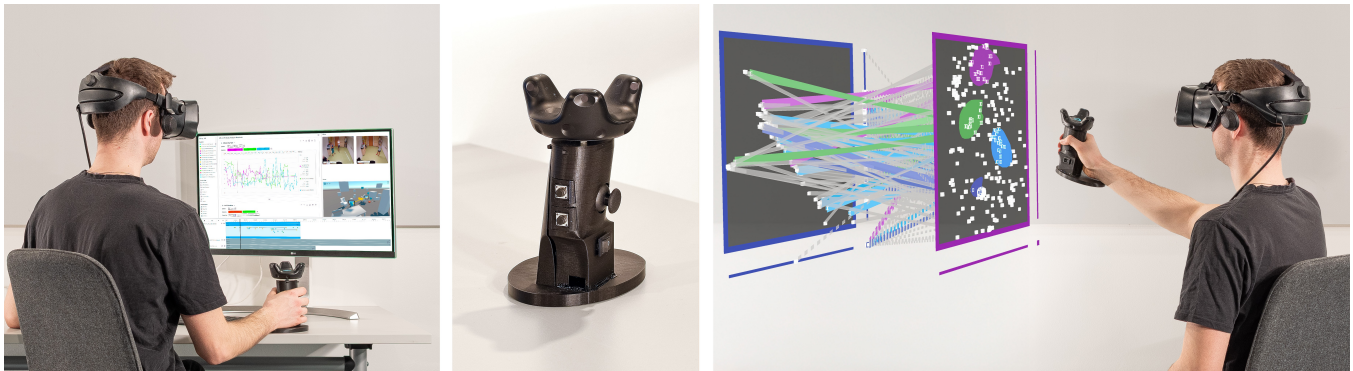
Figure 1: The SpatialMouse combines a desktop mouse with a virtual reality controller, enabling seamless interaction across 2D and 3D information spaces in immersive mixed reality environments.
