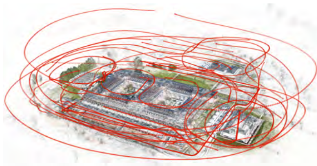
Fig. 18. Uni10K’s sparse point cloud. The scene is reconstructed from more than 10 thousand 4k images at widely varying heights, both from aerial and ground perspective.
