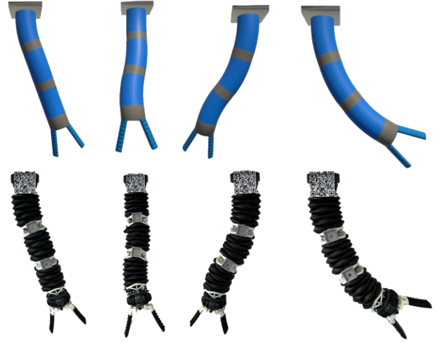
Fig. 7. Comparison of the model visualization (top) with the real soft arm (bottom) in four exemplary poses.
