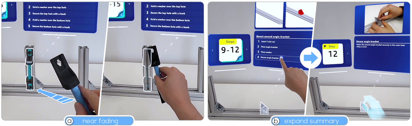
Figure 2: Interaction. (a) Visual occlusion is reduced by fading virtual overlays as the user’s hand approaches the target area. Right: The target outline is preserved to indicate its position. (b) Groups of recurring actions are summarized in structural diagrams that indicate the planned end state. Additionally, our system shows a summarized list of the steps from which the users can jump to the detail view for a specific action, which shows how the actions need to be performed. This enables users to interactively switch between summarized and detailed instructions.
