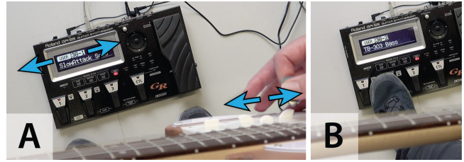
Figure 9: Combining GuitarFins with foot-based interaction. A) Our software sends MIDI commands to the floorboard to quickly and conveniently switch between banks via GuitarFins. B) Patches within the bank can then be switched as usual with the foot while playing.
