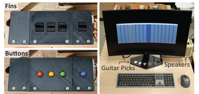
Figure 4: Left: The two devices of our study corresponding to the two conditions C:FINS and C:BUTTONS. Right: The study setup. Participants were seated in front of a screen (during tasks with a guitar and when filling out questionnaires). They could choose from various guitar picks (0.38 mm to 2.0 mm).
