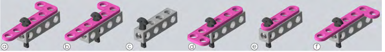
Figure 2: Example of types of errors that can occur during mounting: (a) correct state, (b) mounting screw at the wrong nearby position, (c) omission of the pink hinge, (d) mounting pink hinge in a 180° rotation, (e) mounting an incorrect (but visually similar to the pink hinge) part, (f) mounting the pink hinge in a flipped pose.
